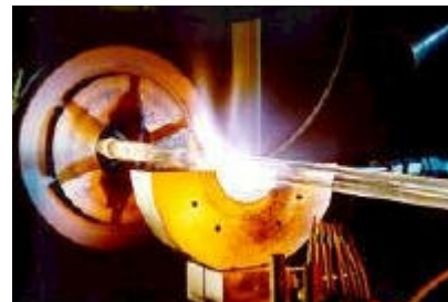
Lathe used in preparing the preform blank
